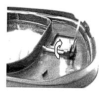
7. Locate new glass over mirror housing. Ensure the spring wire is positioned correctly in its guide track on the housing.
