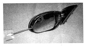
3. Twist the screwdriver to lever the glass from the motor assembly.
